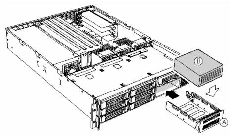
Figure 28: Mounting a Tape Drive
